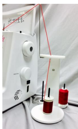
Allowing metallic thread & delicate specialty threads to feed flat.
